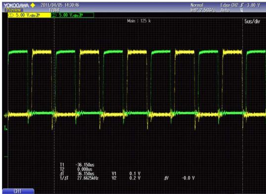
Fig. 5 TL494 output of complementary drive signal waveform
