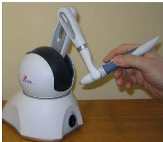
Fig. 4. A PHANTOM Omni force feedback device
