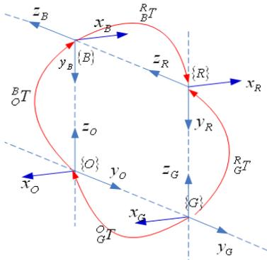
Fig. 7. Coordinate systems coordinate transformations
