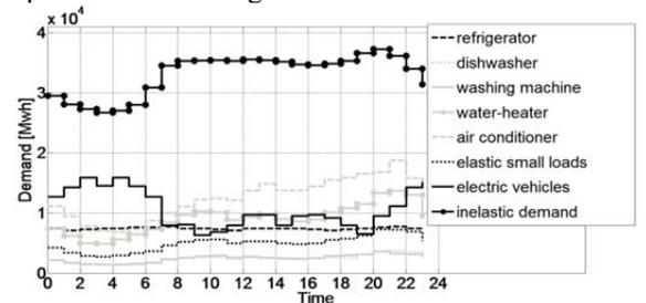
**Figure 1** The typical load curves of each type of domestic appliance
