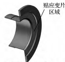
(b) 柔轮及其上贴应变片的区域 (b) Flexspline and the strain gauge cemented area
