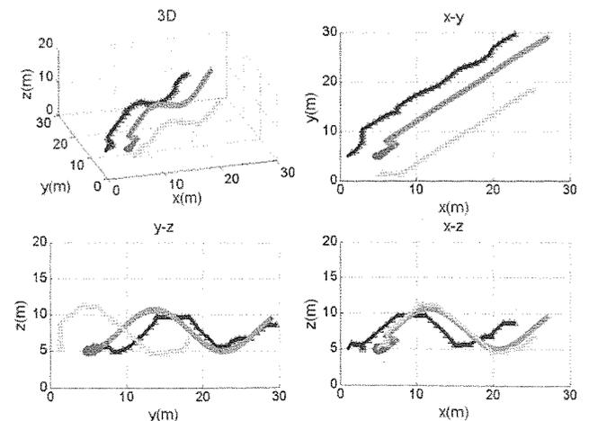
Fig. 7. Simulation result: trajectory and uncertainty set. \*the middle line is the trajectory of the target; the other two lines are the trajectory of the two MVSs, respectively; the blue ellipsoids are the observation result, i.e. the uncertainty sets of the target position at each time instant.
