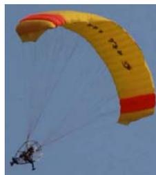
Fig 2. Self-designed soft-wing UAV
