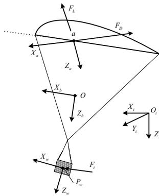
Fig 6. The soft-wing UAV coordinates and its dynamics
