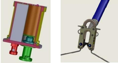
Fig.4 Rope throwing device Fig.5 Lifting lock and carbon fiber rod
