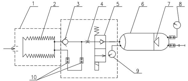
1 - external leakage shell 2 - external bladder 3 - check valve 4 - throttling element 5 - normally closed solenoid valve 6 - pressure hull 7 - internal gas 8 - inflatable gauge 9 - internal pressure gauge 10 - oil-filled connectors
