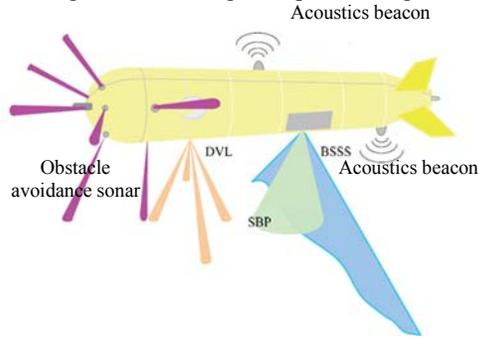
Fig.1 The sensor layout of the Qianlong I
