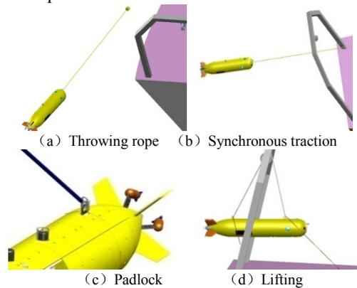
Fig.3 The recovery process of Qianlong I
