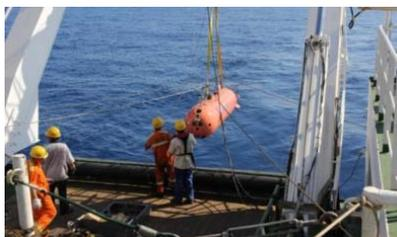
Fig.8 recovery process of the vehicle
