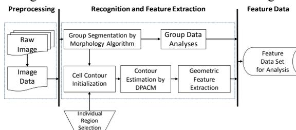
Fig. 3: the automated analysis system for cell patterns cultured on the OEK chip includes three parts: preprocessing, recognition and feature extraction and feature data combination.
