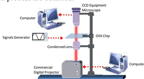
Fig. 1: the schematic illustration of the optically-induced electrokinetics (OEK) experimental setup for generating the PEGDA patterns.
