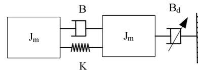
Fig. 6. Mass-spring-damper model of robot joint with MR damper
