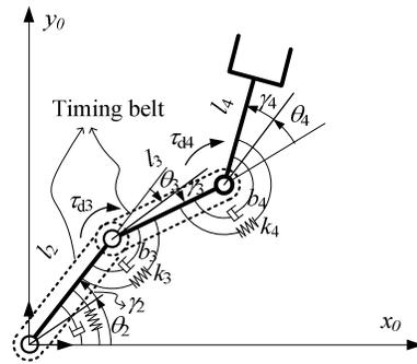
Fig. 2 Model of robot including joint elasticity
