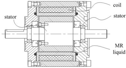
Fig. 5. Structure of variable viscous rotational MR damper
