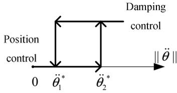
Fig. 4. Switching sketch with hysteresis of joint control between low damping state and high damping state
