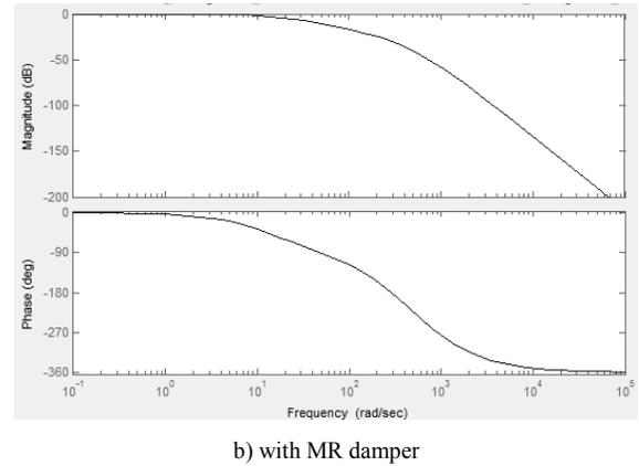
Fig. 8. Frequency response of robot joint
