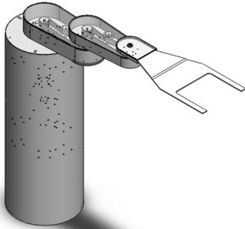
Fig. 1. Structure of SCARA robot
