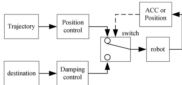
Fig. 3 Switching control system
