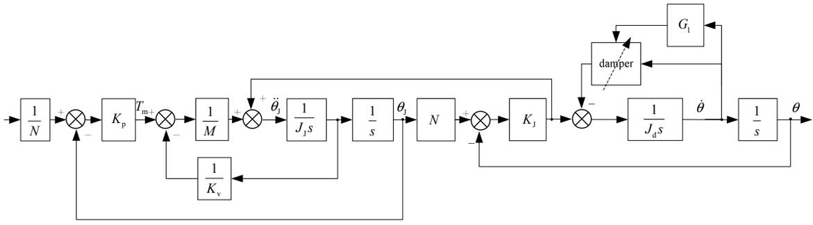
Fig. 7. Block diagram of robot joint transfer function
