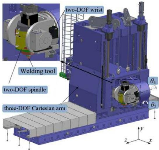
Figure 3 Design of the two-DOF wrist
