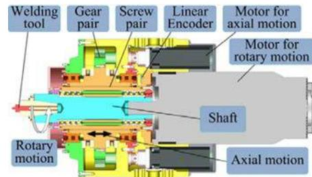
of welding tool, and the linear encoder is used to position the axial movement. The motor for rotary motion is adopted to drive the shaft directly and achieve rotary movement of welding tool, and the encoder on the motor implements stirring speed feedback. The two DOFs are independent and orthogonal.
