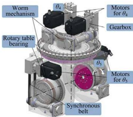
provide precise angular position feedback. With such a structure, the drive capability can be enhanced for heavy load, and the motion accuracy of the wrist can be improved using dual pinion anti-backlash drive technology (Kwon *et al.*, 2004).
