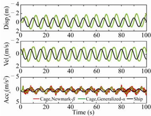
Fig. 11. Vertical displacement, velocity and acceleration of ship and cage at the depth of 5000 m with sinusoidal ship motion and depth-dependent ocean current.
