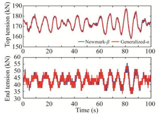
Fig. 9. Dynamic tension at both ends of umbilical cable at the depth of 5000 m with only ship motion.
