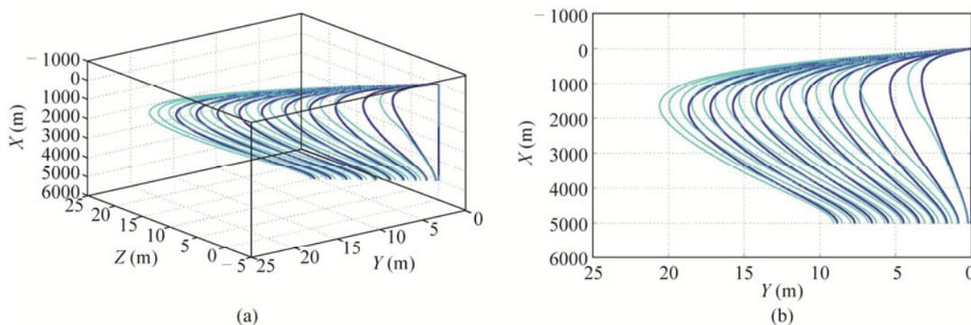
**Fig. 10.** (a) Three-dimensional dynamic configurations every other 100 time steps within 100 s using the generalized- $\alpha$  method (solid bold blue line) and Newmark- $\beta$  (solid cyan line) at 5000 m, and (b) projections in  $XOY$  plane.
