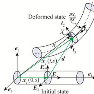
Fig. 2. Cable kinematics in a three-dimensional space.
