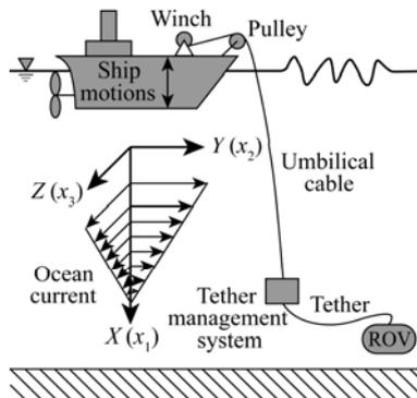
Fig. 1. A schematic of a typical deep-sea ROV system.
