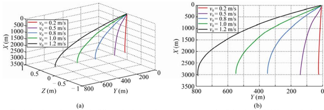
Fig. 4. Steady configurations in different depth-dependent ocean currents at the diving depth of 3000 m, (a) the three-dimensional configurations, and (b) projections in XOY vertical plane.
