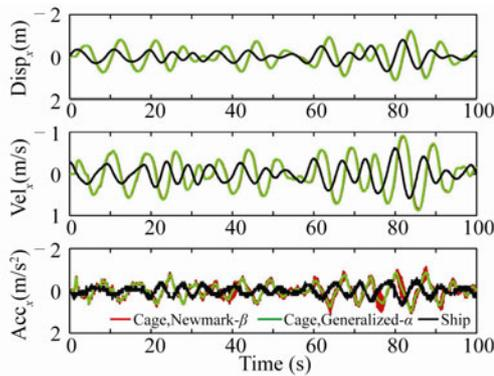
Fig. 8. Vertical displacement, velocity and acceleration of ship and cage at the diving depth of 5000 m with only ship motion.
