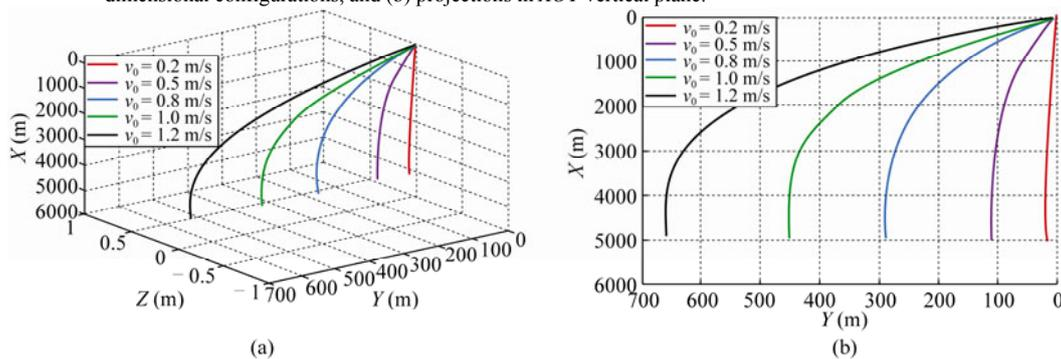
Fig. 5. Steady configurations in different depth-dependent ocean currents at the diving depth of 5000 m, (a) the three-dimensional configurations, and (b) projections in XOY vertical plane.
