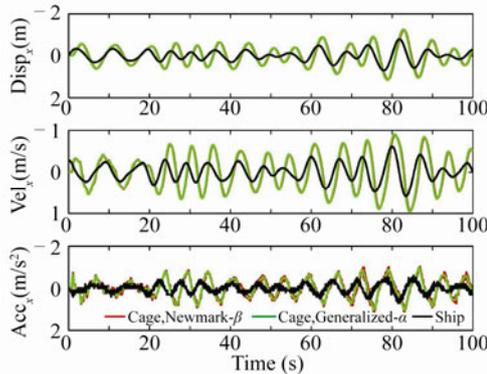
Fig. 6. Vertical displacement, velocity and acceleration of ship and cage at the diving depth of 3000 m with only ship motion.
