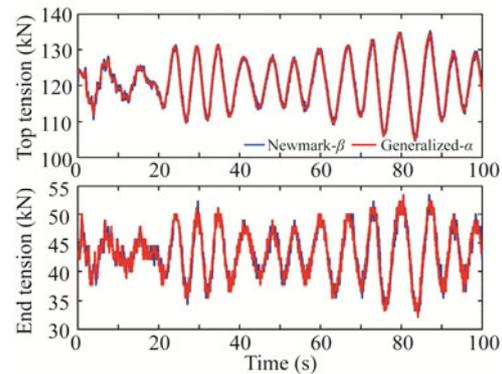
Fig. 7. Dynamic tension at both ends of the umbilical cable at the depth of 3000 m with only ship motion.
