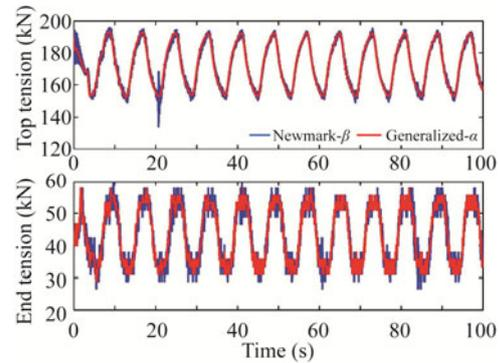
Fig. 12. Dynamic tension at both ends of the umbilical cable at the depth of 5000 m with sinusoidal ship motion and depth-dependent ocean current.
