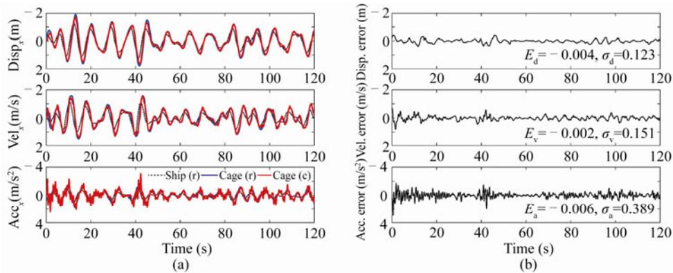
**Fig. 3.** (a) Comparison of cage motion between the calculated and the measured results, and (b) corresponding motion errors within 120 s. In (a), the black dash line is the measured motion of the supporting ship, the blue solid line is the measured motion of cage, and the red solid line is the calculated motion of the same cage by using the presented geometrically exact formulation.
