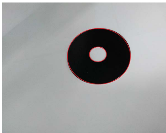
图 12 椭圆检测 Fig.12 Ellipse detection
