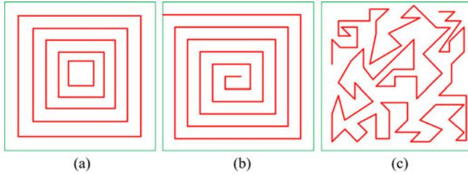
Fig. 4. The scanning strategies in AFM imaging. The red lines denote the AFM tip scanning trajectory on the sample surface and the green square is the boundary of the local image to be scanned. (a) The square scanning strategy; (b) The spiral scanning strategy; (c) The optimal scanning strategy.
