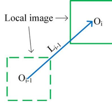
Fig. 3. Method to determine the center of the local imaging after one step of manipulation. The dashed block and solid block denote the range of last local imaging and the current local imaging, respectively, and the bold line with the arrow denotes the moving vector for the last step of manipulation.
