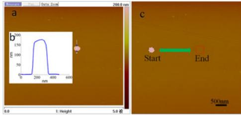
Fig. 6. The goal image and object recognition. (a) The goal image with the size of  $5 \times 5 \mu\text{m}$ ; (b) The profile of the nanoparticle of interest with a diameter of 200 nm; (c) The image with an object recognized. The black dotted circles denote the object at the starting location, while the red solid square box is the destination location.
