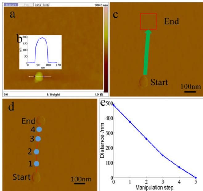
Fig. 9. The tracking process of nano-manipulation of a virus (a) The goal image with the size  $1 \times 1 \mu\text{m}$ ; (b) The profile of one virus of interest in the image (a), and the diameter of the virus is less than 100 nm; (c) The image with one virus recognized. The red solid box is the destination location; (d) The tracking process of manipulation of the virus; (e) The distance between the virus and the destination location at each step of manipulation.
