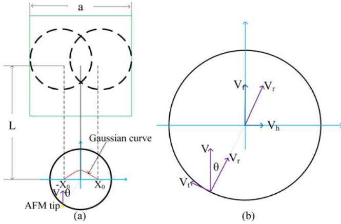
Fig. 2. The calculation of the manipulation distance and the local imaging range. (a) The locations of the object by one step of manipulation. The solid circle denotes the current location of the object, and the dashed circles denote the possible location of the object after one step of manipulation. Green box is the boundary of local image to be acquired; (b) The kinematic model of the target object during manipulation.
