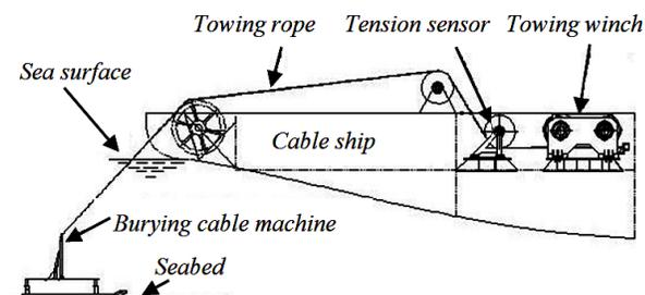
Fig. 1. The towing winch in the sea cable burying system
