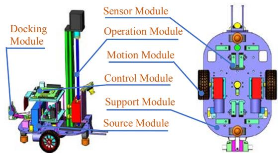
Fig.6 3D Prototype of Handbots
