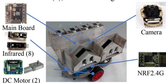
Fig.10 Control system of Transbots
