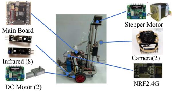
Fig.8 Control system of Handbots
