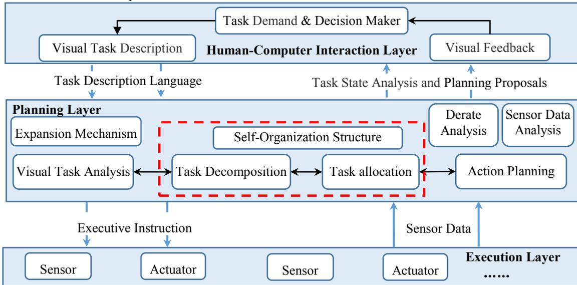
Fig.5 System structure of SociBuilder system
