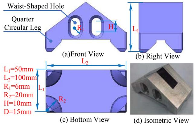
Fig.3 Structure of Rof-module
