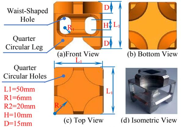
Fig.2 Structure of Squ-module
