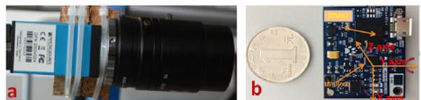
Fig. 3. The system modality: (a) the wearable monocular camera; (b) our designed IMU
