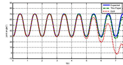
Fig. 7. The comparison between the actual trajectories and the expected trajectory of Joint 2
