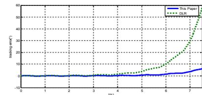
Fig. 10. The tracking errors of Joint 2
