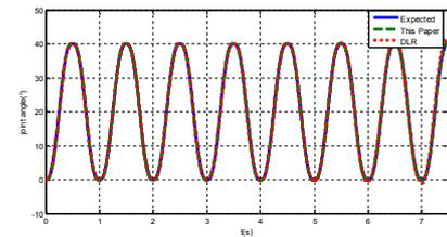
Fig. 8. The comparison between the actual trajectories and the expected trajectory of Joint 3
