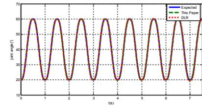
Fig. 6. The comparison between the actual trajectories and the expected trajectory of Joint 1
