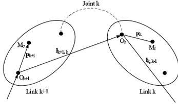
Fig. 1. The details between adjacent rigid bodies in the model of spatial operator algebra
