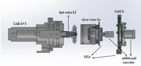
Fig. 2. The rotor-separated model of the k-th flexible joint
