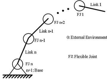
Fig. 3. The schema of a series flexible-joint manipulator with n DoFs based on FS-SEA
