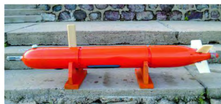
图 1 中国科学院沈阳自动化所研制的便携式 AUV Fig. 1 The portable AUV made by Shenyang Institute of Automation Chinese Academy of Sciences
