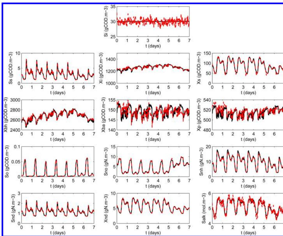
**Figure 3.** Trajectories of the actual process state (solid lines) and the estimates given by the distributed EKF (dashed lines) of reactor 1 under dry conditions.
