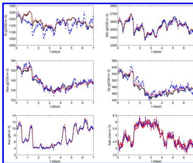
**Figure 5.** Trajectories of the actual process state (solid lines) and the estimates given by the EKF (dashed lines) and the distributed EKF (dash-dotted lines) of reactor 4 under rain conditions.
