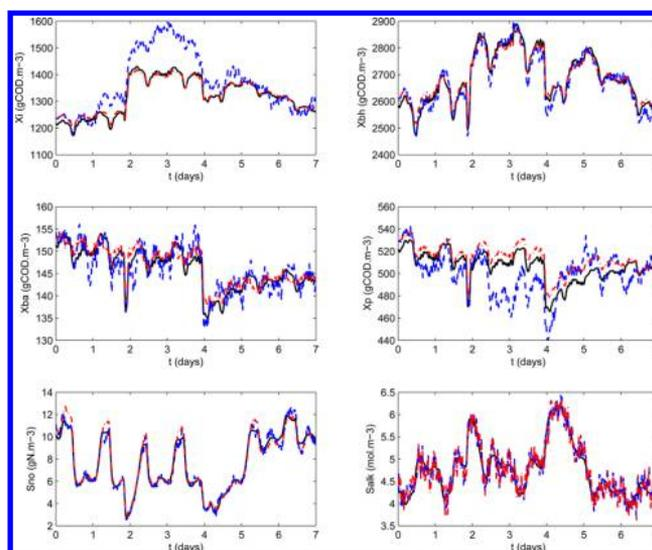
**Figure 6.** Trajectories of the actual process state (solid lines) and the estimates given by the EKF (dashed lines) and the distributed EKF (dash-dotted lines) of reactor 4 under storm conditions.
