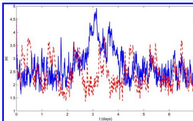
**Figure 4.** Trajectories of the Euclidean norm of normalized estimation errors given by the EKF (solid lines) and the distributed EKF (dashed lines) under dry conditions.
