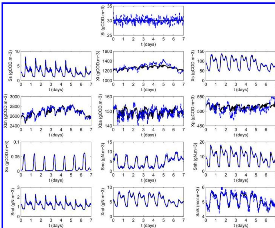
Figure 2. Trajectories of the actual process state (solid lines) and the estimates given by the EKF (dashed lines) of reactor 1 under dry conditions.
