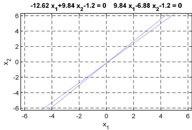
It is seen that the intersection point of the two lines is very close to origin point, which means the amplitude of the input initial state is small, so the controller will output smaller actions.
