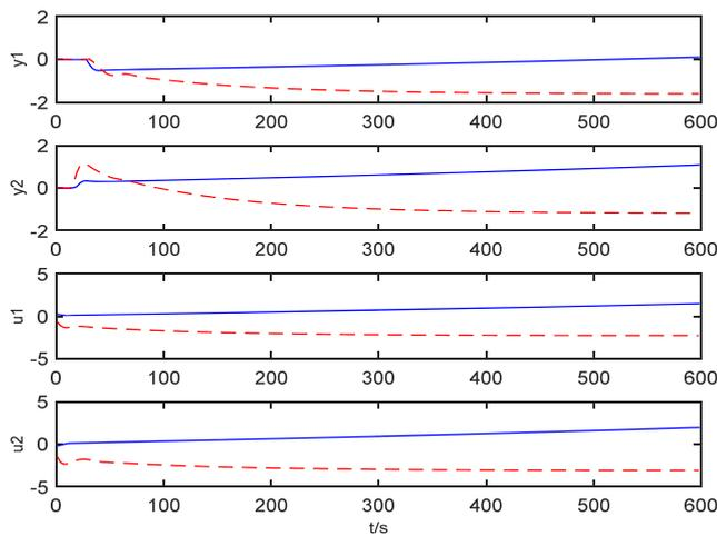
**Figure 15** Control effect comparison between modified model and unmodified model under mismatch mode 2 and set point two (see online version for colours)
