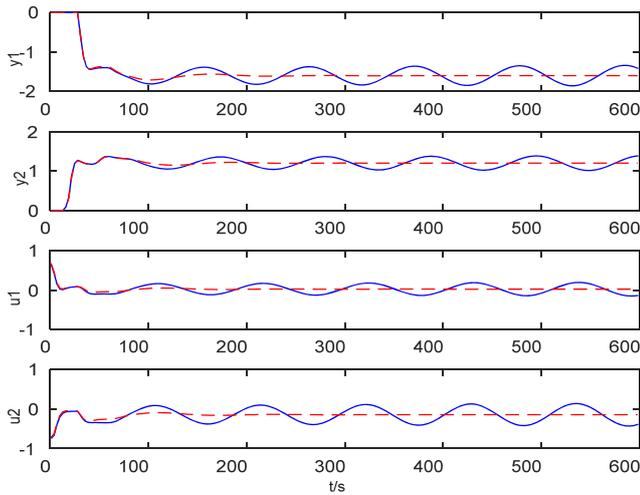
**Figure 14** Control effect comparison between modified model and unmodified model under mismatch mode 2 and set point one (see online version for colours)
