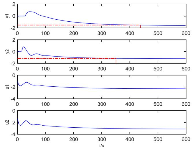
This paper uses the standard DMC algorithm to do the simulation experiments, the relevant parameters are as following. The set point one is  $[-1.6, -1.2]^T$ , set point two is  $[-1.6, 1.2]^T$ , and will use in all of simulation. The weight coefficient matrix  $Q, R$  are chosen to be a unit diagonal matrix (take this value for all), the input and output curves are shown in Figure 2.
