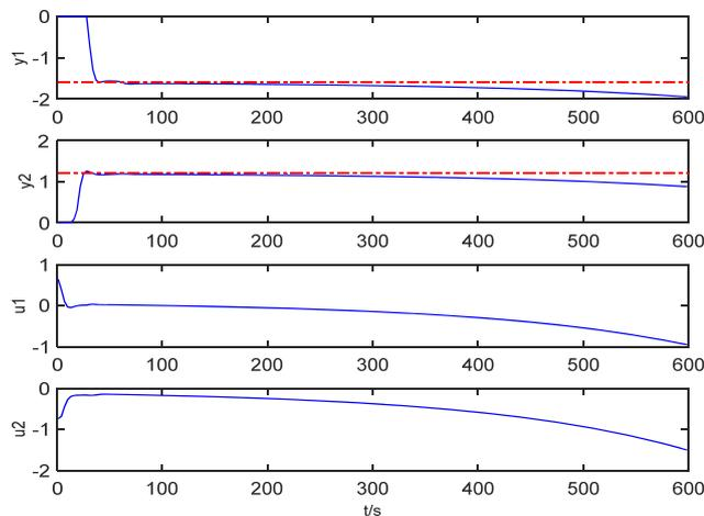
From Figures 6 and 7, it can be seen that the output of the two sets of the mismatch is not to reach the set point, the mismatch causes the controller action is too large, so that the divergence of input and output curve is observed finally. When the moving direction of the two set points is changed, the condition number of the matrix is also changed, which leads to the change of the degree of the model morbidity.
