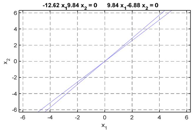
It is seen that the intersection point of two straight lines is the origin point, it means output initial state which corresponding to input initial state is  $[0, 0]^T$ .
