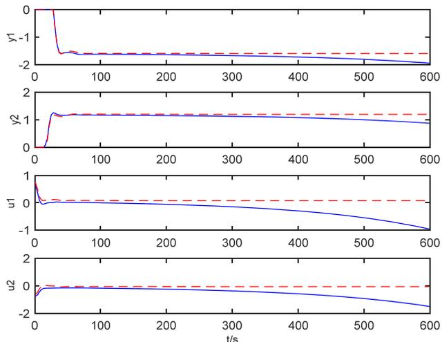
Using set point 1 and set point 2 to simulate under the mismatch mode 1 and mode 2, the control effects are shown as Figures 12 to 15.
