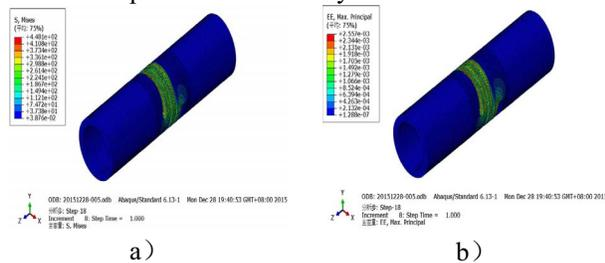
Fig. 6. Stress distribution and elastic deformation of different elastic components under an axial load of 1N
