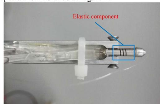
Fig. 2. The integrated prototype elastic component
