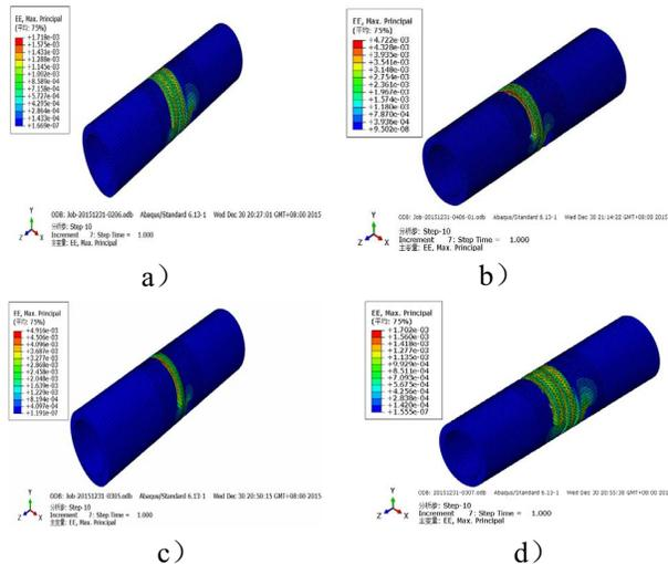
Fig. 8. Elastic deformation of different elastic components under a axial load of 1N
