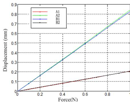
Fig. 9. Relation between deformation and the force of different sizes under a axial load of 1N
