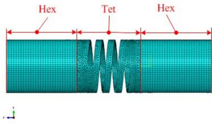
Fig. 3. The distribution of mesh controls
