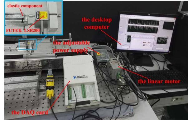
Fig. 4. The experiment equipment platform
