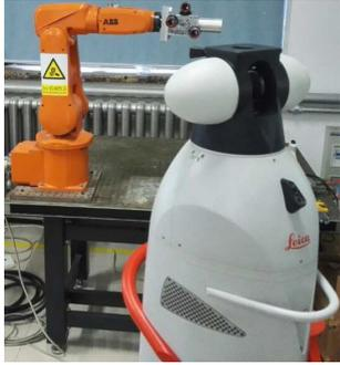
Fig. 6. The laser tracker used for kinematics evaluation
