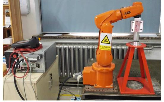
Fig. 5. The prototype of LfD-based assembly robot
