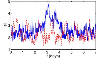
Fig. 4. Trajectories of the Euclidean norm of normalized estimation errors given by the EKF (solid lines) and the distributed EKF (dashed lines).
