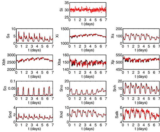
Fig. 3. Trajectories of the actual process state (solid lines) and the estimates given by the distributed EKF (dashed lines) of reactor 1.
