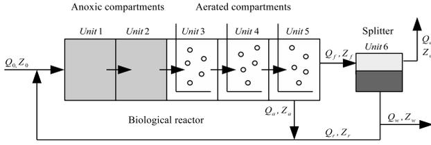
Fig. 1. General overview of the modified BSM1.
