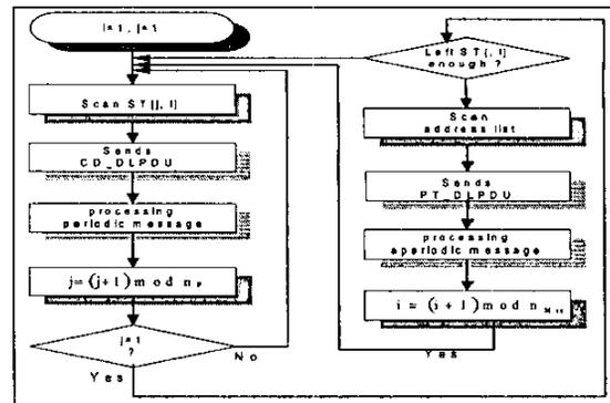
Fig.1 Procedure of LAS sending CD and PT
