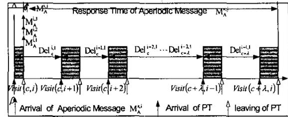
Fig.6. Response procedure of an aperiodic message
