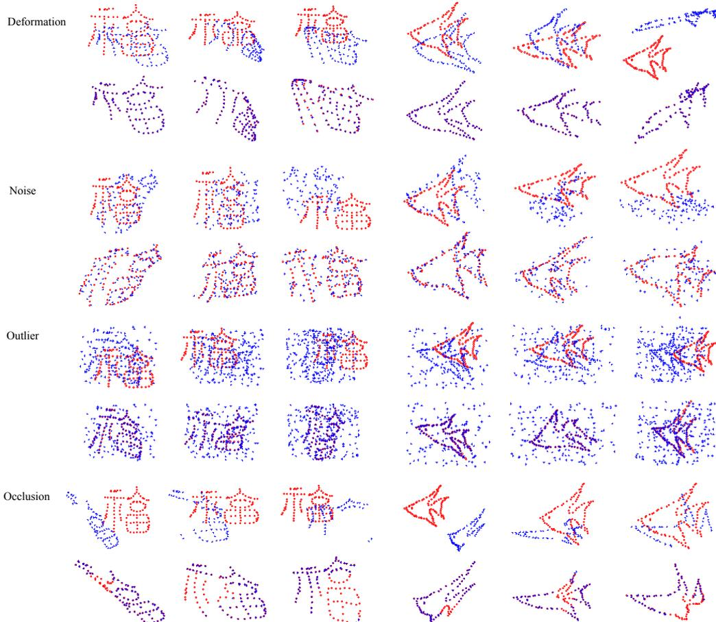
Figure 2. Registration results with our method on the Chinese character (left) and fish (right) patterns. From left to right are degradations of two types of in three different levels. The mission is to align the model point set (red circles) onto the scene point set (blue pluses).
