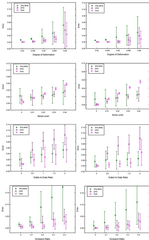
Figure 3. Quantification of the proposed algorithm compared to TPS-RPM [20] and CPD [3] on the corresponding datasets. Right column: the shape of fish. Left column: the shape of a Chinese character. Each error bar indicates the registration error mean and the standard deviation over 100 runs.
