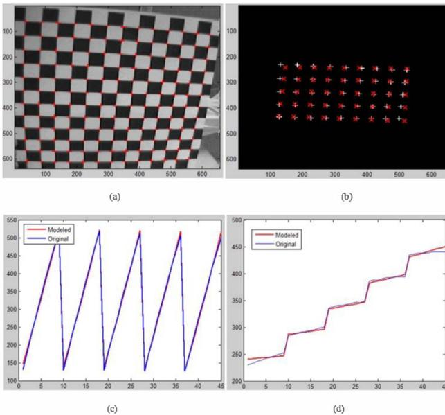
Figure 4. Illustration of camera calibration pattern modeling: (a) Captured calibration pattern; (b) Modeled points against the original points; (c) Modeled and original  $x$  coordinates; (d) Modeled and original  $y$  coordinates.
