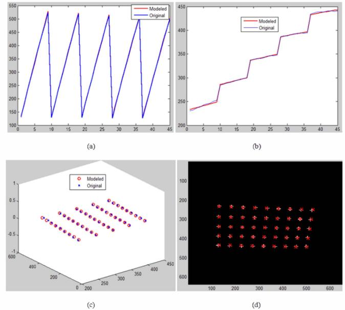
Figure 6. Illustration of camera calibration pattern modeling with another found center: (a) Modeled and original  $x$  coordinates; (b) Modeled and original  $y$  coordinates; (c)-(d) Modeled points against the original points.
