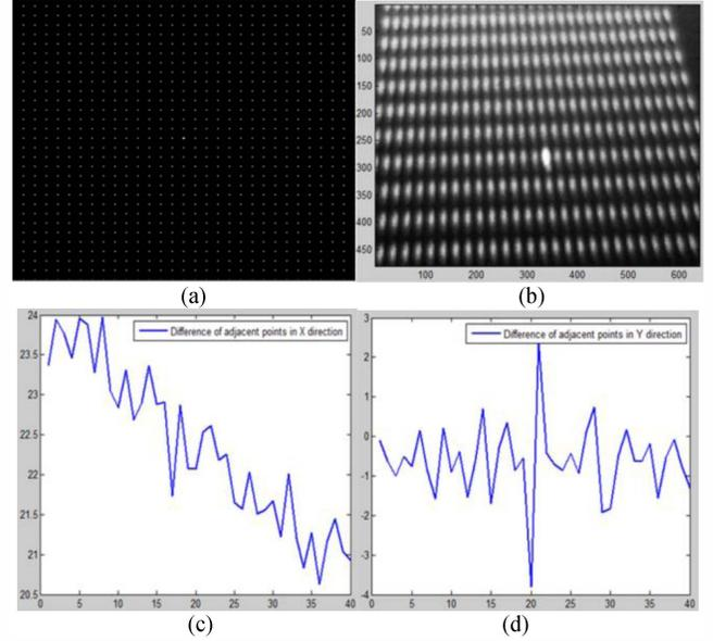
Figure 1. Illustration of noise; (a) Designed pattern; (b) Captured pattern; (c) plot of the  $x$  coordinate differences in pixels; (d) plot of the  $y$  coordinate differences in pixels. (The  $y$  axis label is mm and  $x$  axis label is index number for (c) and (d))
