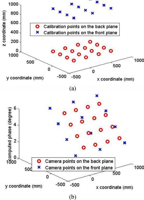
Figure 5. Two sets of points used for calibration: (a) Designed points in the virtual space  $(X_i^w, Y_i^w, Z_i^w)$   $i = 1, \dots, 28$ ; (b) Computed points
