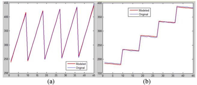
Figure 3. Results of modeling the pattern in the camera view (Fig. 1 (b)) with the searched projection center (a) Modeled and original  $x$  coordinates; (b) Modeled and original  $y$  coordinates.
