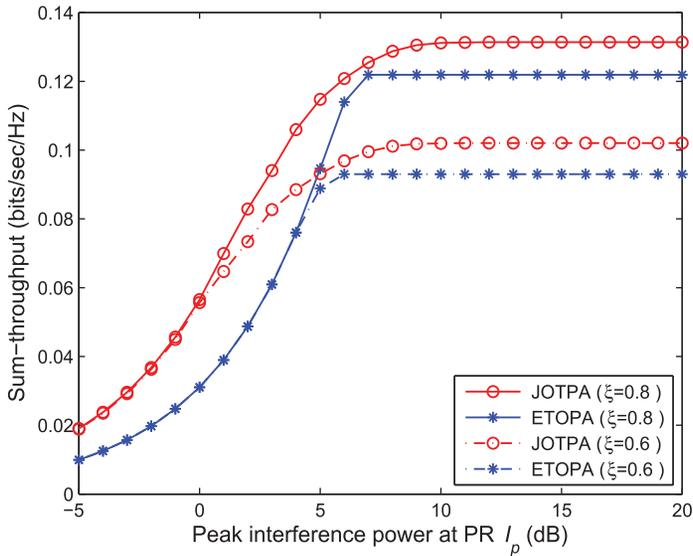
Fig. 6. Sum-throughput versus the peak interference power at PR for JOTPA and ETOPA with different energy conversion efficiencies in Deployment 1.
