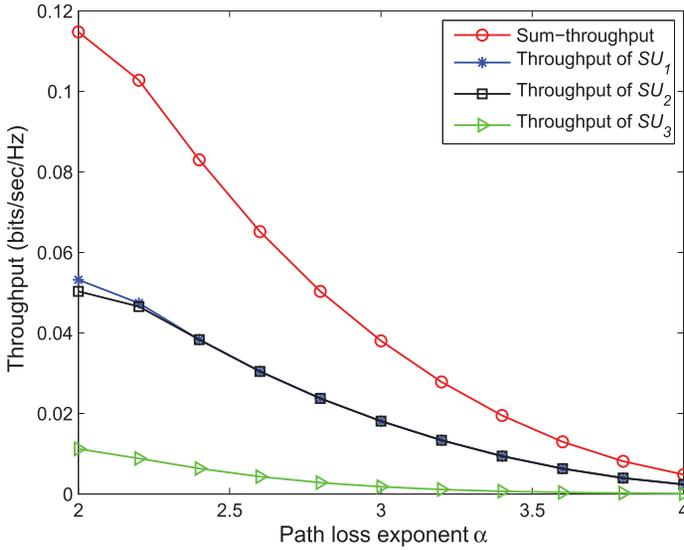
Fig. 5. Throughput versus path loss exponent in Deployment 1.
