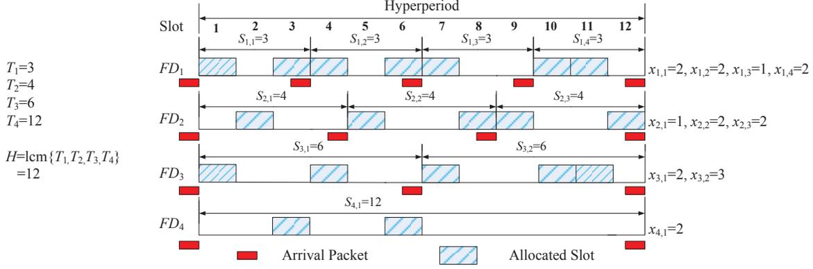
Figure 3. Example of slot allocation in one hyperperiod
