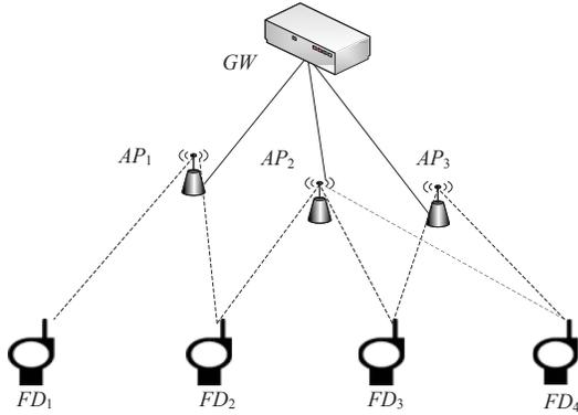
Figure 2. An example of a redundant star topology
