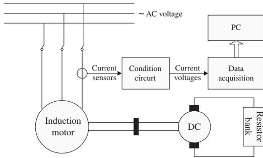
Fig. 3. Schematic of the experimental test rig
