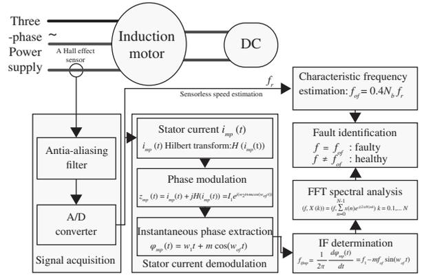
Fig. 2. Schematic diagram of the proposed bearing outer raceway fault detection method
