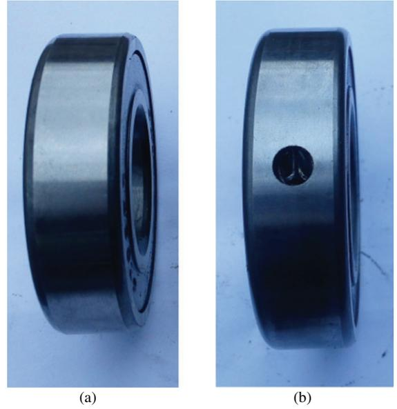
Fig. 5. Tested bearings: (a) Healthy (b) outer raceway fault
