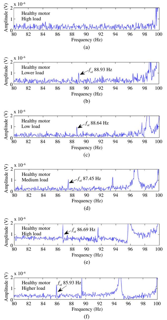
Fig. 10. FFT spectra of the instantaneous frequency under six different tests: high loaded healthy motor, and motor with outer raceway fault under five different load conditions: (a) High loaded healthy motor (b) lower load (c) low load (d) medium load (e) high load (f) higher load
