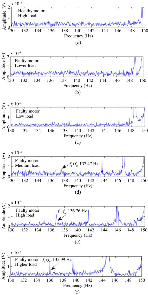
Fig. 9. FFT spectra of the stator current under six different tests: high loaded healthy motor, and motor with outer raceway fault under five different load conditions: (a) High loaded healthy motor (b) lower load (c) low load (d) medium load (e) high load (f) higher load
