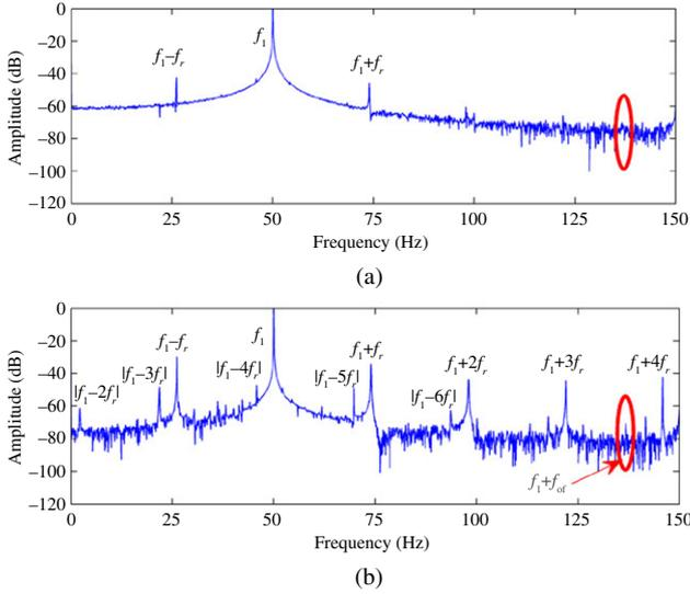
Fig. 6. FFT spectra of the stator current (0–150 Hz) under high-load condition: (a) Healthy IM (b) IM with bearing outer raceway fault
