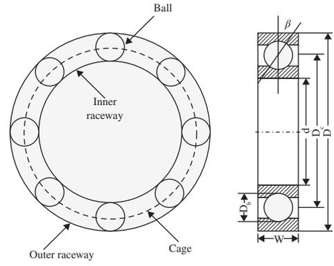
Fig. 1. Typical structure of a rolling-element bearing with main parameters
