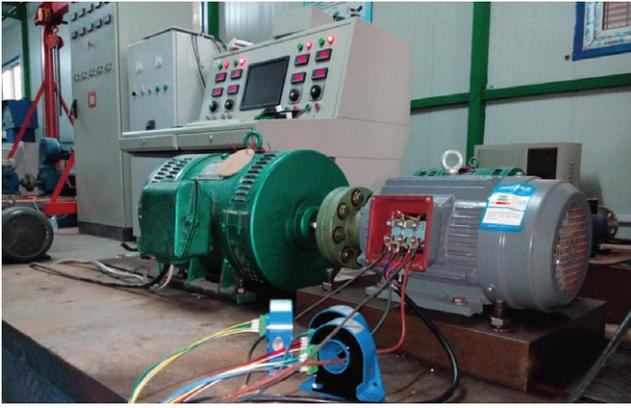
Fig. 4. Photograph of the experimental setup used for bearing fault detection
