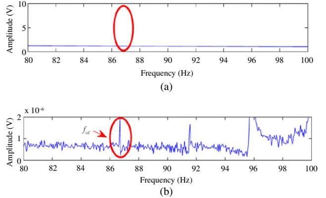
Fig. 8. Frequency-domain signals (0–0.2 s) under high-load condition: (a) Instantaneous phase (b) IF of the stator current in a faulty induction motor
