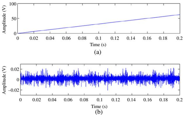
Fig. 7. Time-domain signals (0–0.2 s) under high-load condition: (a) Instantaneous phase (b) IF of the stator current in a faulty induction motor
