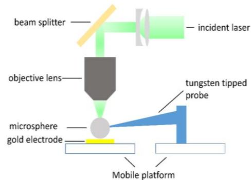
Figure 1. Schematic of entire experimental photonic nanojet-based laser-processing system.
