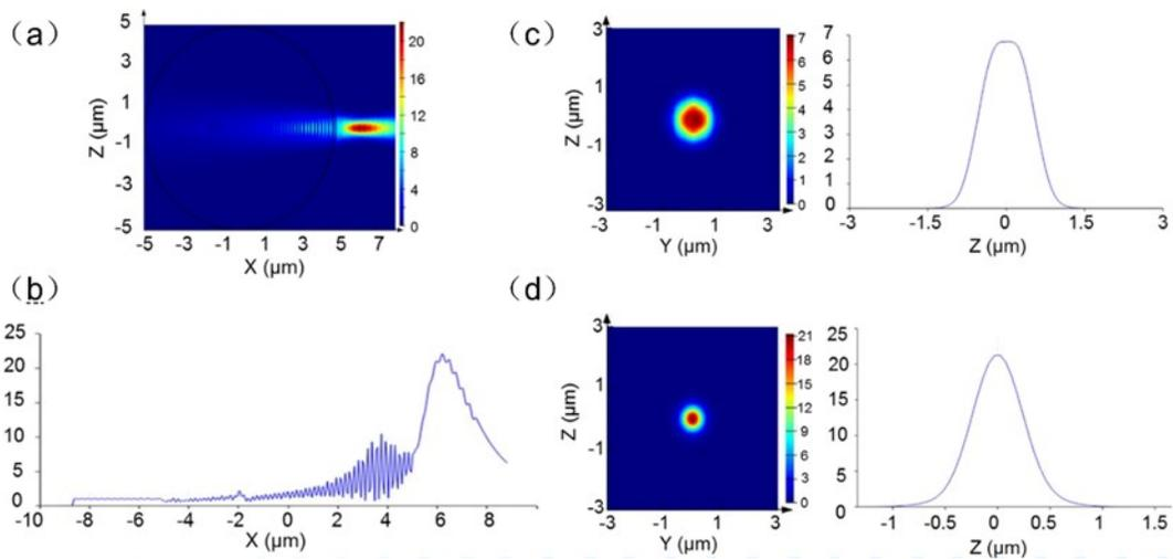
Figure 2. (a) Simulation results for silica microsphere 10  $\mu\text{m}$  in diameter. (b) Intensity distribution along x-axis of (a). (c) Simulation results showing intensity on material surface. (d) Simulation results for plane of photonic nanojet at peak intensity.
