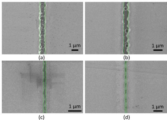
Figure 3. SEM images of specimens processed at laser power of 120 mW and platform moving rates of (a) 5  $\mu\text{m}/\text{s}$ , (b) 10  $\mu\text{m}/\text{s}$ , (c) 15  $\mu\text{m}/\text{s}$ , and (d) 20  $\mu\text{m}/\text{s}$ . Scale bars represent 1  $\mu\text{m}$ .
