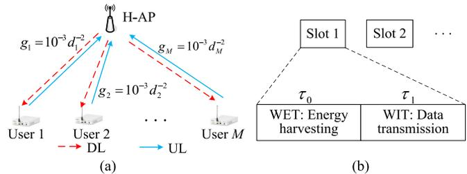
Fig. 1. System model. (a) Network architecture. (b) Slot architecture.
