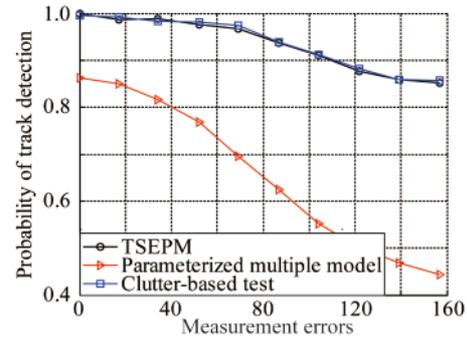
Fig. 7. Probability of the track detection ( $P_D$ ) with variable measurement errors.
