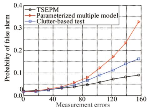
Fig. 8. Probability of the false alarm ( $P_F$ ) with variable measurement errors.
