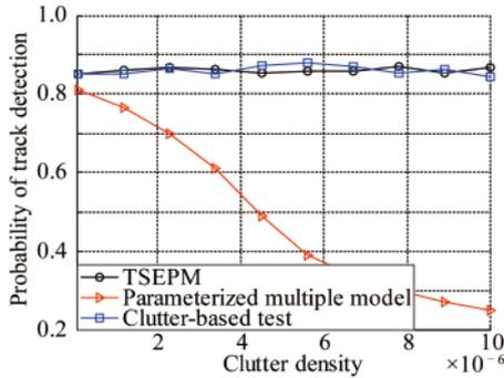
Fig. 5. Probability of the track detection ( $P_D$ ) with variable clutter density.
