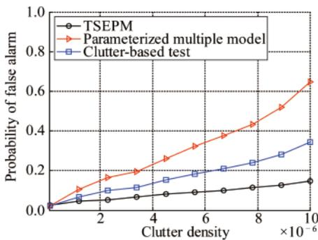
Fig. 6. Probability of the false alarm ( $P_F$ ) with variable clutter density.
