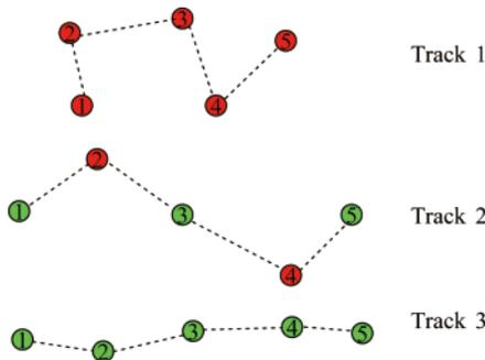
**Fig. 1.** Nonnegligible influence on the track initiation process generated by heavy clutter. Red and green circles indicate the clutter and measurement derived from targets, respectively. The number means time. Thus, Track 1 is a false alarm, Track 3 is a true track, and Track 2 is a semi-correct track.
