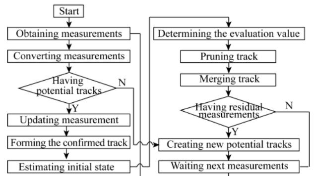
Fig. 4. Flow diagram of the TSEPM method for the track initiation problems.
