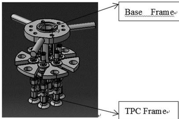
Figure 5. The TPC Frame and Base Frame of tool head.
