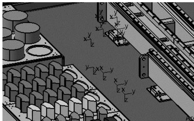
Figure 4. The distribution point group of robots.
