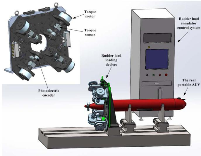
Fig. 7. Mechanical structure of the rudder load simulator
