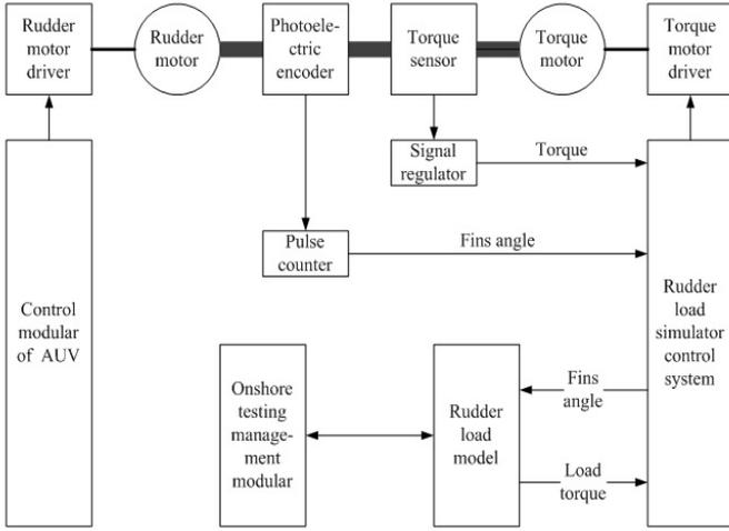
Fig. 5. Architecture of the rudder load simulator
