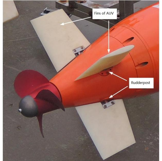
Fig. 4. Rudder system of the Explorer-100 AUV
