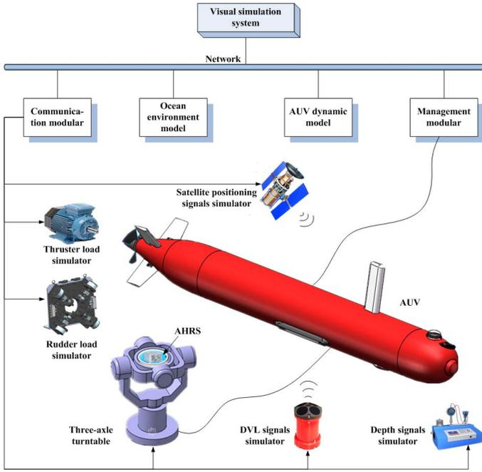
Fig. 1. Architecture of the onshore testing system for AUV
