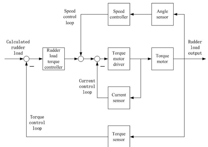
Fig. 6. Control diagram of the rudder load simulator
