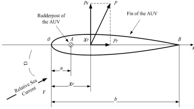
Fig. 2. Sketch top view of the fin of AUV
