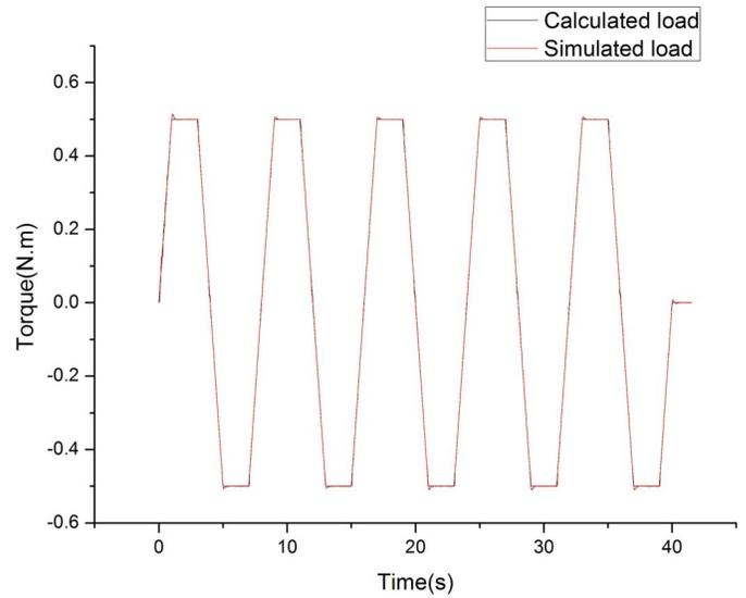
Fig. 9. simulated load with a trapezoidal change calculated load (max 0.5N.m)
