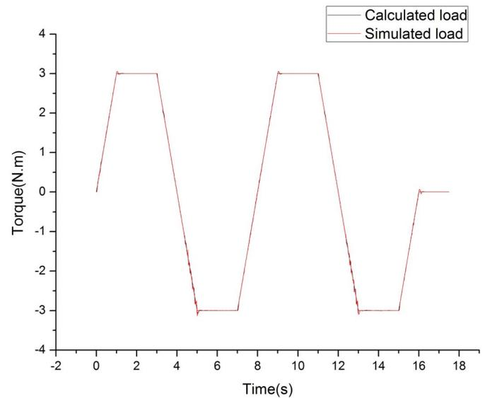
Fig. 10. simulated load with a trapezoidal change calculated load (max 3N.m)
