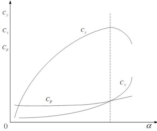
Fig. 3. Illustration of the variation relationship between non-dimensional coefficients of the fin
