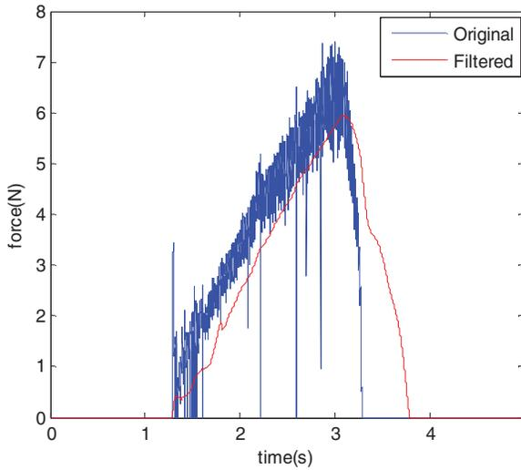
Fig.9 Contact force after low pass filtered
