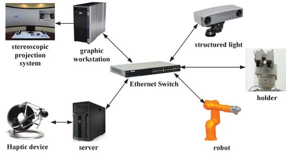
Fig.1 Experiment platform
