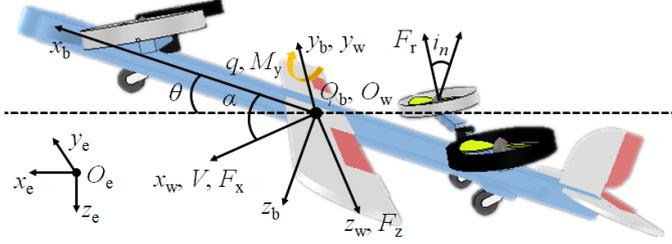
Fig. 1. Quad-TRUAV and coordinate systems
