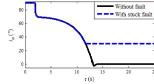
Fig. 8. Curve of rotor-tilt angle with  $30^\circ$  stuck fault
