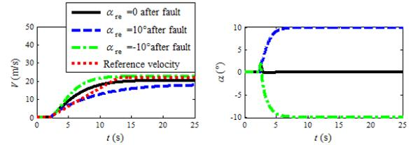
Fig. 9. Curves of  $V$  and  $\alpha$  with different  $\alpha_{\text{re}}$  after  $70^\circ$  rotor-tilt axle stuck fault
