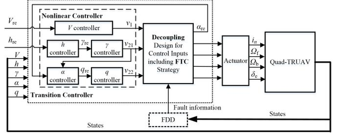
Fig. 2. Transition controller structure
