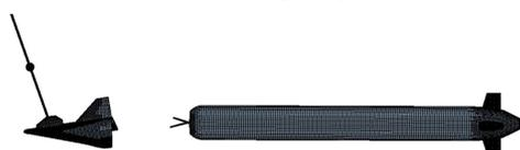
Fig 10. Grid model of AUV and the V-shaped wing
