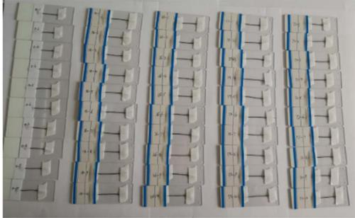
Fig. 5. Specimen of the magnet wires with different degraded status for optical observation.
