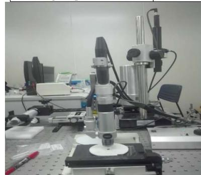
Fig. 3. Optical microscope measurement platform.
