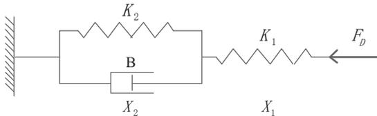
Fig. 2 The schematic diagram of Kelvin-Boltzmann model
