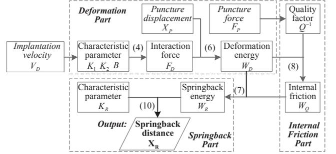
Fig. 4 The flow diagram of acquiring the springback displacement. The italic texts in the box represent the three elements which should be got to calculate the springback displacement based on the three models. The numbers on the connecting lines represent the equation number above.
