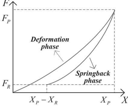
Fig. 3 The relation between displacement and force in two phases
