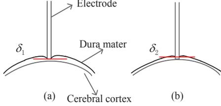
Fig. 1 The schematic diagram of two phases in electrodes implantation through dura mater. (a) The critical state of the puncture of the dura mater. (b) The moment of the puncture occurs and the dura mater springs back.
