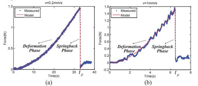
Fig. 12 The validation results of the models in two phases by two velocities ((a)  $v=0.2\text{mm/s}$ , (b)  $v=0.4\text{mm/s}$ )
