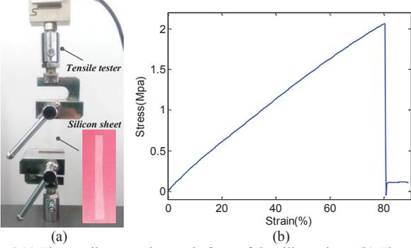
Fig. 6 (a) The tensile strength test platform of the silicon sheet, (b) The stress-strain curve of the tensile strength test
