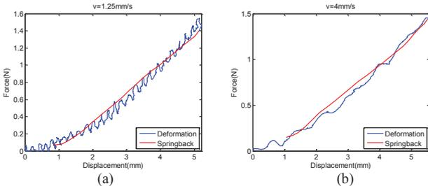
Fig. 10 The variation of the force and the displacement in deformation phase and springback phase ((a)  $v=1.25\text{mm/s}$ , (b)  $v=4\text{mm/s}$ )
