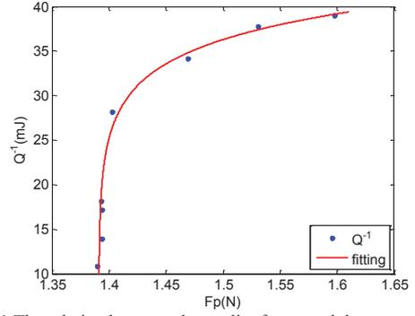
Fig. 11 The relation between the quality factor and the puncture force
