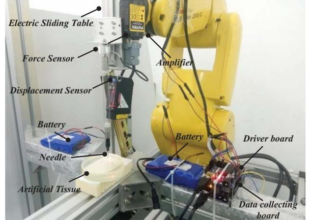
Fig. 5 The implantation experiment platform
