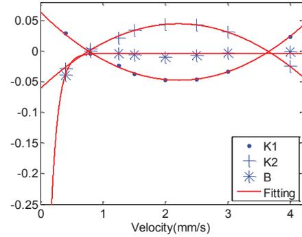
Fig. 8 The fitting results between KB model parameters and the velocity
