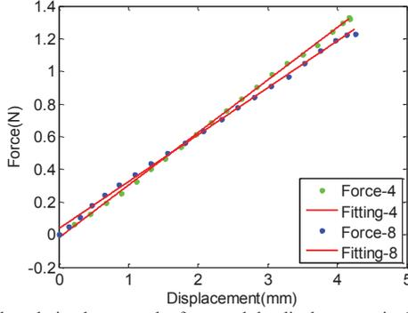
Fig. 9 The relation between the force and the displacement in the springback phase. The numbers in the legend represent the velocity numbers in TABLE I
