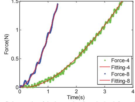
Fig. 7 The fitting results of the interaction force in the deformation phase. The numbers in the legend represent the velocity numbers in TABLE I
