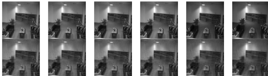
Figure 4. Background rereconstruction with illumination changes, the first row: 6 consecutive frames, the second row: the results of background rereconstruction
