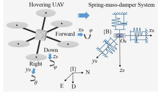
Figure 4. A hovering UAV acts as a spring-mass-damper system.
