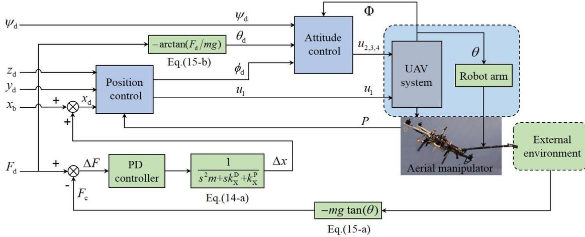
Figure 6. Contact force control block diagram of aerial manipulator.
