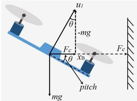
Figure 5. Relationships among contact force, thrust and gravity force.
