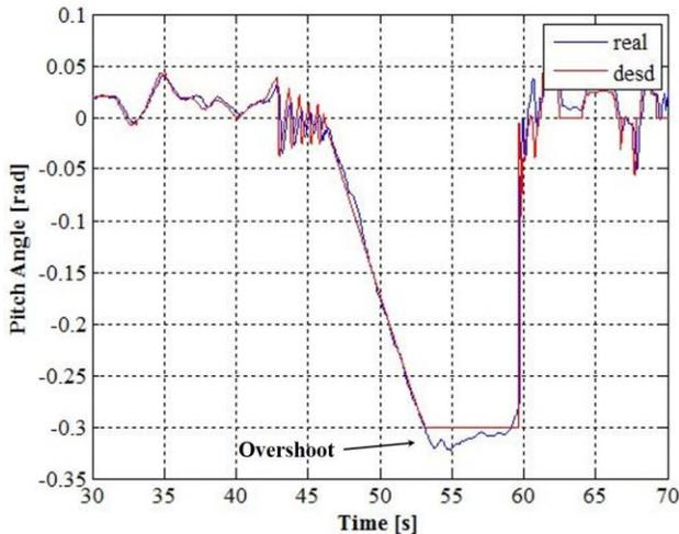
Figure 10. The pitch angle states of UAV in the operation process.
