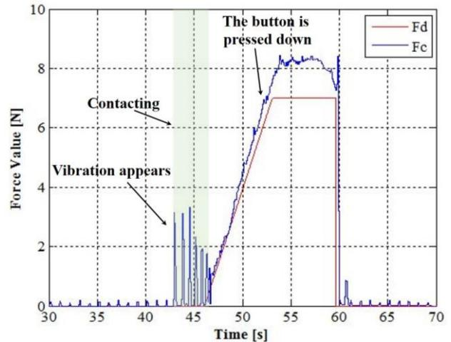
Figure 9. The measured contact force and desired force.
