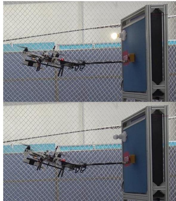
Figure 1. An aerial manipulator is pressing the emergency switch to turn off the light.
