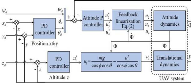
Figure 3. Control block diagram of UAV system.
