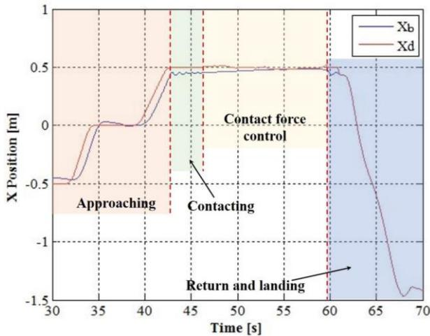
Figure 8. The real-time X position of aerial manipulator.
