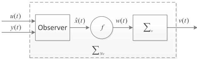
Fig. 1. Nonlinear system for calculating  $v(t)$ .
