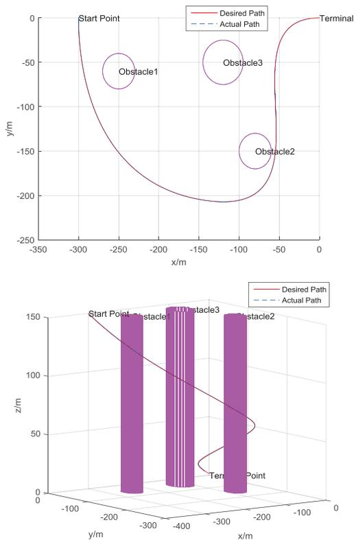
Fig. 10 Actual result of trajectory following in SIMULINK
