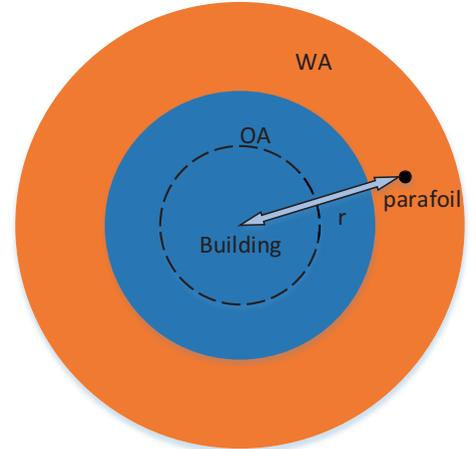
Fig. 3 Area description for parafoil obstacles avoidance
