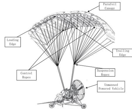
Fig. 1 Structure of parafoil system
