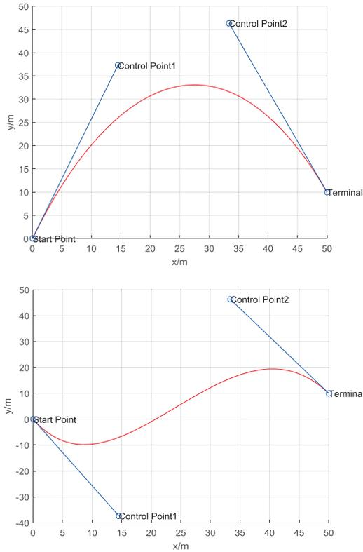
Fig. 3 Single cubic Bezier curve
