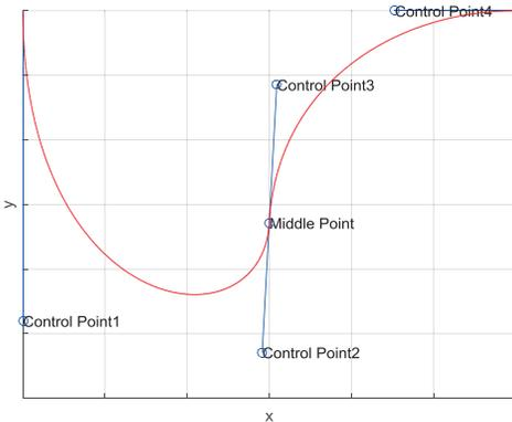
Fig. 5 Guidance path with two Bezier curves
