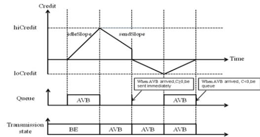
Fig. 1. Credit Based Shaping(CBS) Algorithm
