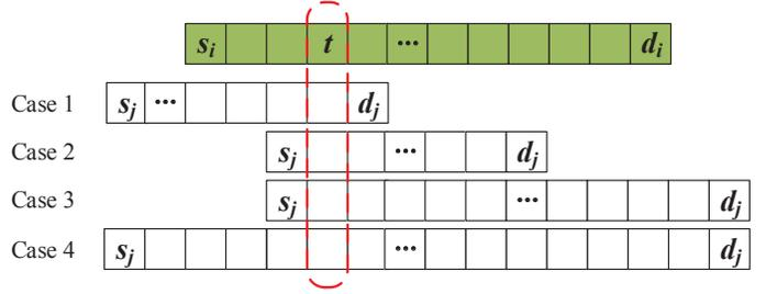
Fig. 5. Four cases of lifetime relationship between  $L_i$  and  $L_j$
