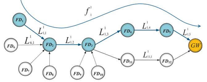
Fig. 1. Mesh topology in IWSNs
