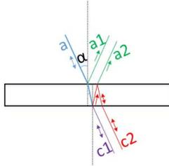
Fig. 3. Optical path of the laser beam passing through the glass sample.
