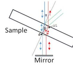
Fig. 5. Optical path within the glass, when the emerging beam is not perpendicular to the glass surface.
