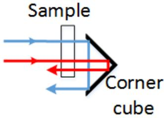
Fig. 2. Optical path of the emerging beam when the sample doesn't cover the corner cube completely.
