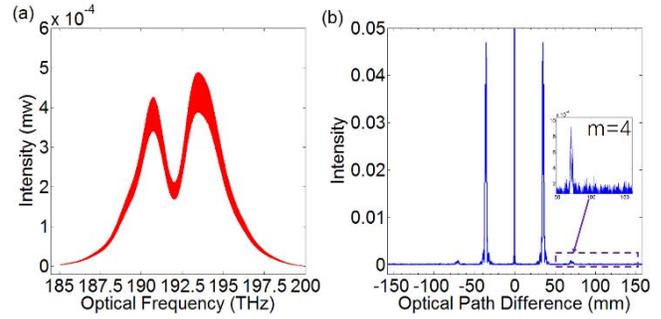
Fig. 6. (a) The interference signal of the angle measurement (the angle of incidence is about 12°). (b) Fourier-transformed signals of the spectrum.
