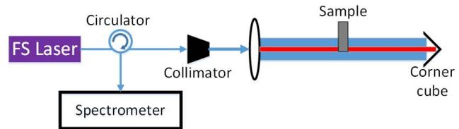
Fig. 1. Schematic of the setup for the glass-thickness measurement.
