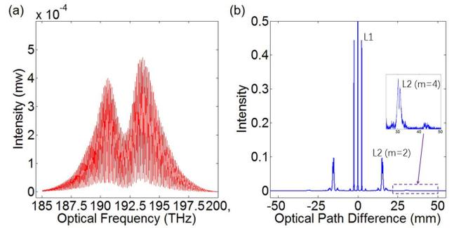
Fig. 4. (a) Interference signal of the glass-thickness measurement. (b) Fourier-transformed signals of the spectrum ( $m$  denotes the number of times the beams are reflected within the sample).
