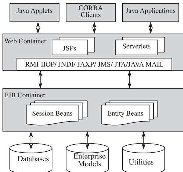
Figure 3. Generic ERP framework based on J2EE.
