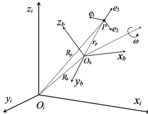
Figure 2. Geometry of an inertial frame, a body frame, and an accelerometer frame.
