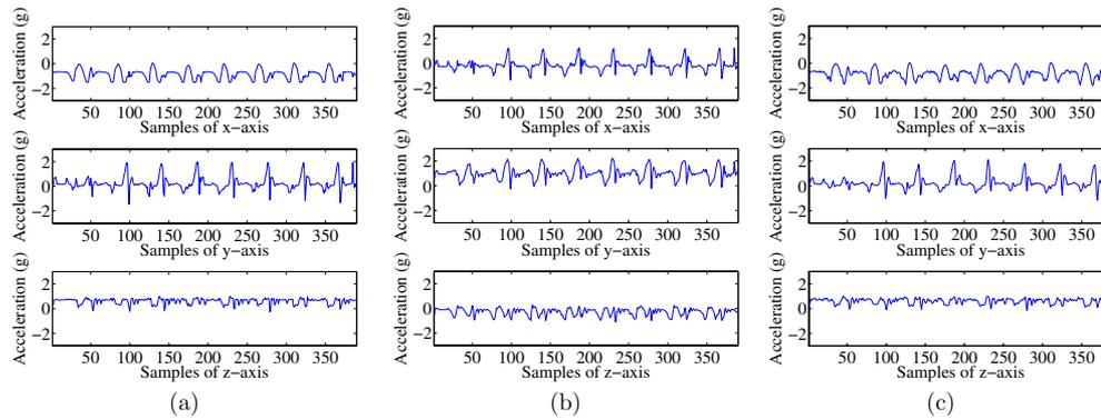
**Figure 5.** A period of ‘cycling’ signals produced from a left-shank-mounted accelerometer. (a) No installation error. (b) Both installation errors. (c) After eliminating orientation errors.
