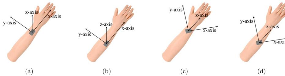
**Figure 1.** An arm-mounted accelerometer. (a) No installation error. (b) Misplacement. (c) Orientation error. (d) Both installation errors.
