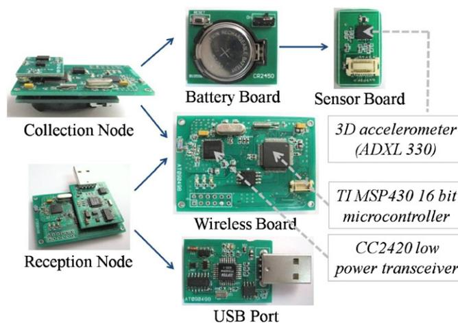
Figure 4. Configuration of the collection node and the reception node.
