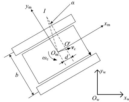
Fig. 1 Platform of the vehicle undergoing general planar motion.
