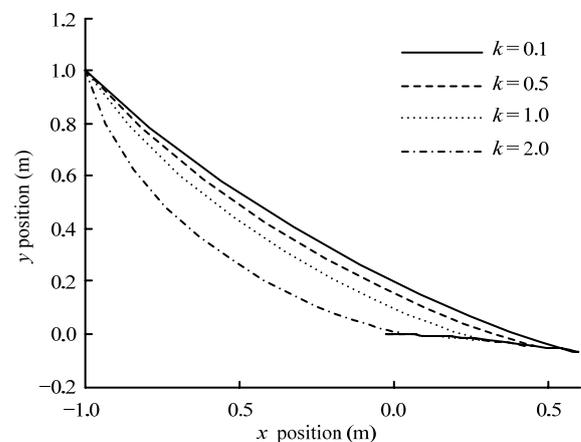
Fig. 4 Trajectories of  $x$  via  $y$  with different slipping coefficient.
