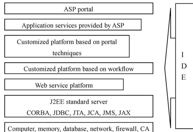
Figure 2. ASP platform architecture.
