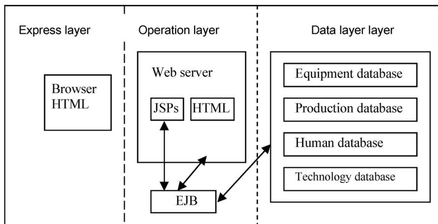
Figure 3. System architecture based on J2EE.
